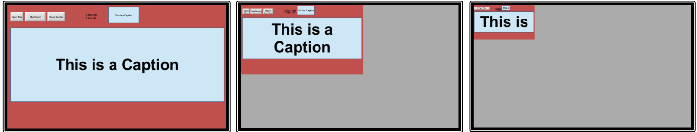
Figure 8: Three images of a resized screen. The Viewer Module is not resized (grey area), but the screen is resized using the Open() function. (The screen is closed before the new Open() function is called). The option is set to resize the objects on the screen, however, note that the text is not resized. Text size is a function of the size of the Graphics Module ( viewer.exe )
