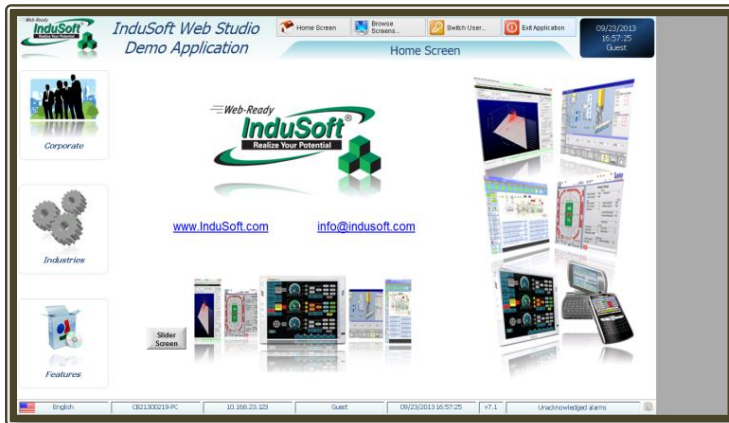
Figure 7: The InduSoft "PC Demo" application is natively built in 1280x800 resolution (5:3 or 1.6 aspect ratio). It is shown displayed on a 1366x768 monitor (16:9 or 1.67 aspect ratio) on the left, and a 1024x768 monitor (4:3 or 1.3 aspect ratio) on the right. The application is Auto-scaled to fit maximized in the monitor at either the Y-Max (left picture) leaving extra X space on the monitor, or X-Max (right picture) leaving extra Y space on the monitor.
