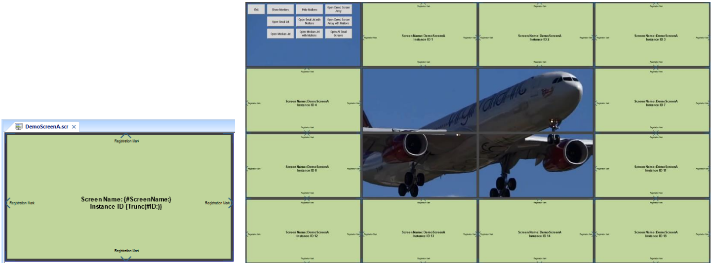
Figure 13: Single Demo Screen showing mullions and registration marks. Pushbuttons located on the main screen with mullions added (underneath the Demo Screen popups) open the screens or screen groups. Screens are closed by clicking on them.
